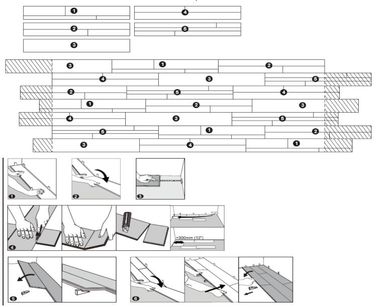
1. First row, first plank: After thoroughly cleaning the subfloor, you should begin laying from left to right. Position the first plank so that grooved edge is facing you. Place the floorboard 1/4'' / 6 mm from the left wall. Use spacers between the wall and the floorboard.
