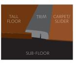
**END CAP** (often times called Square Edge or Threshold) is most commonly used when butting up to carpet or a sliding glass door.
